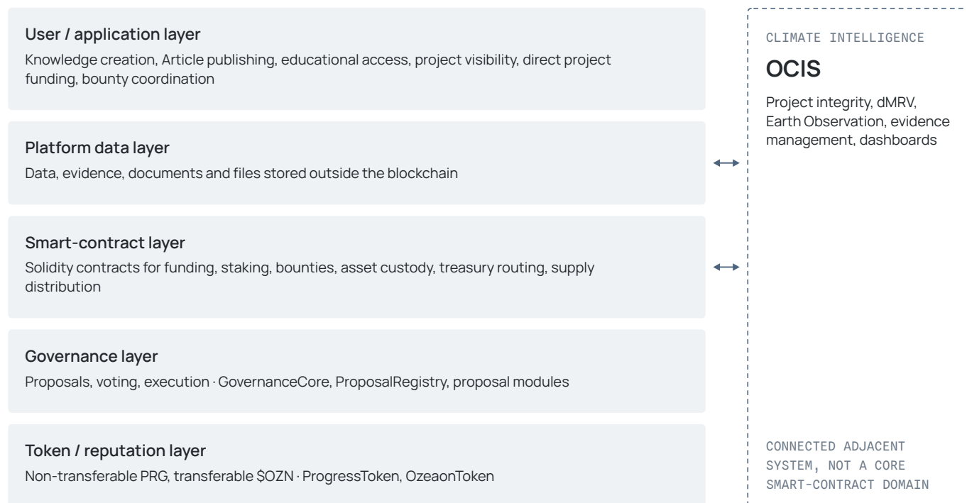
FIGURE 4.1 — OZEAON SYSTEM ARCHITECTURE OVERVIEW
